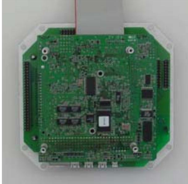
*Athena CPU with IDE cable mounted on stack*
