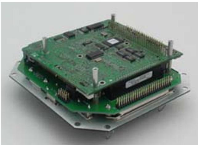
*Athena CPU board mounted on panel board*
