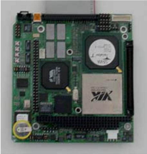
*Athena CPU with IDE cable installed*
