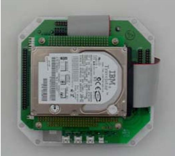
*Hard drive mounted onto stack*
